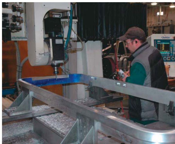
Top: 3D CAD design Middle: Assembly start Bottom: CnC frame machining
